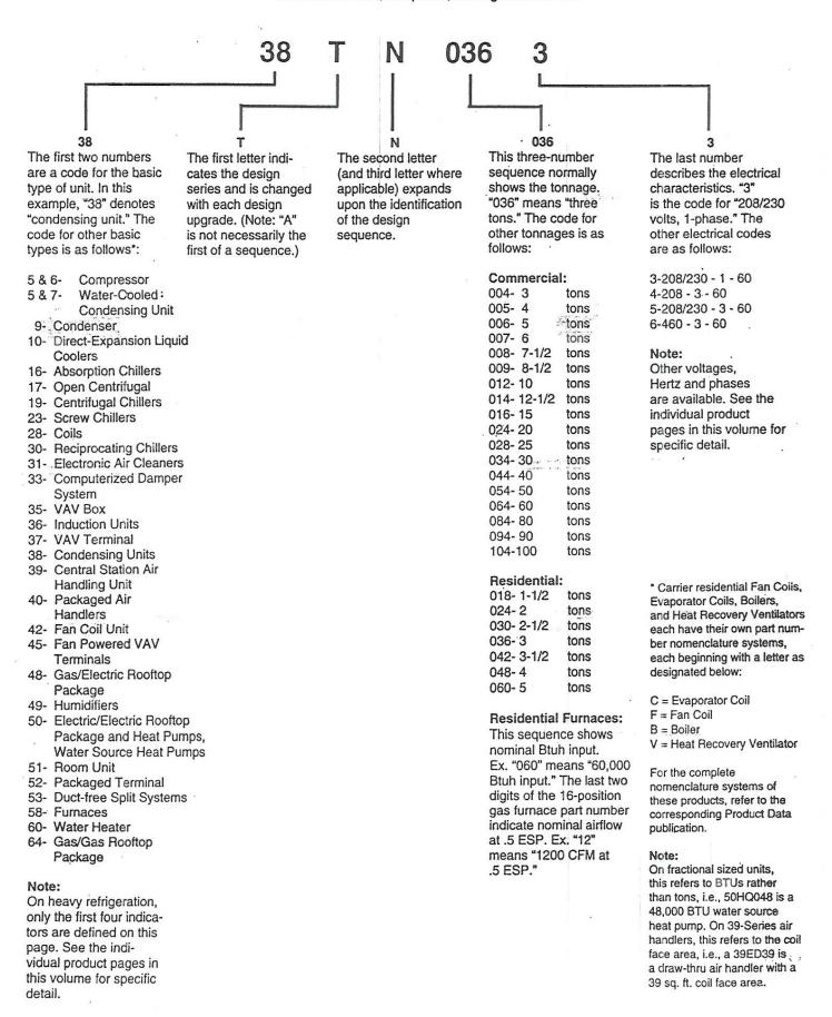
Each Carrier product is identified by a series of numbers and letters that are designed to quickly and easily communicate the major characteristics of the product. Exceptions to this designation may be determined from the product data. For example, a sixty-ton gas/electric rooftop package, 208/230 volts, three-phase, is designated like this:
