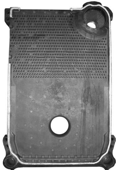
Figure 7: Affixing the Fiberglass Rope
