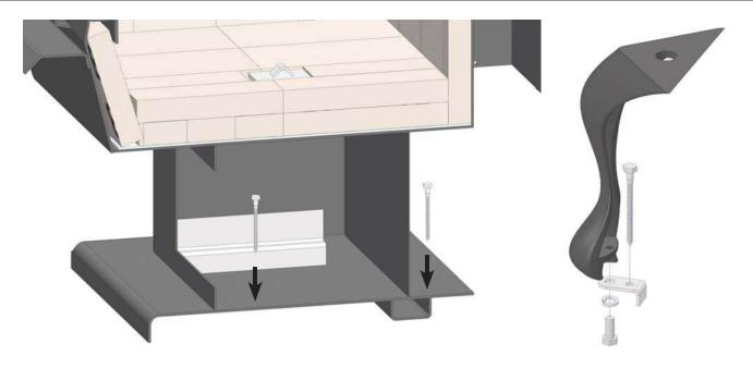
In mobile home installations, the stove must be securely fastened to the floor using the tie-downs provided in the Outside Air kit. (For the pedestal model, remove the ash drawer to access the screw down holes. For the Leg model, use the Leg Anchor Kit (P/N ZR8039) to secure stove to floor.)
