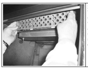
2. Once you remove the flame shield, you'll find the combustor. The honeycomb combustor can be made of different materials such as cordierite, mulite or even stainless steel. They are all the same with regard to removal and caution should be taken so as to not drop or damage the combustor. If your combustor has never been cleaned according the manufacturers directions, you may wish to clean the combustor before replacing it with a new combustor, see "CATALYTIC COMBUSTOR CLEANING".
