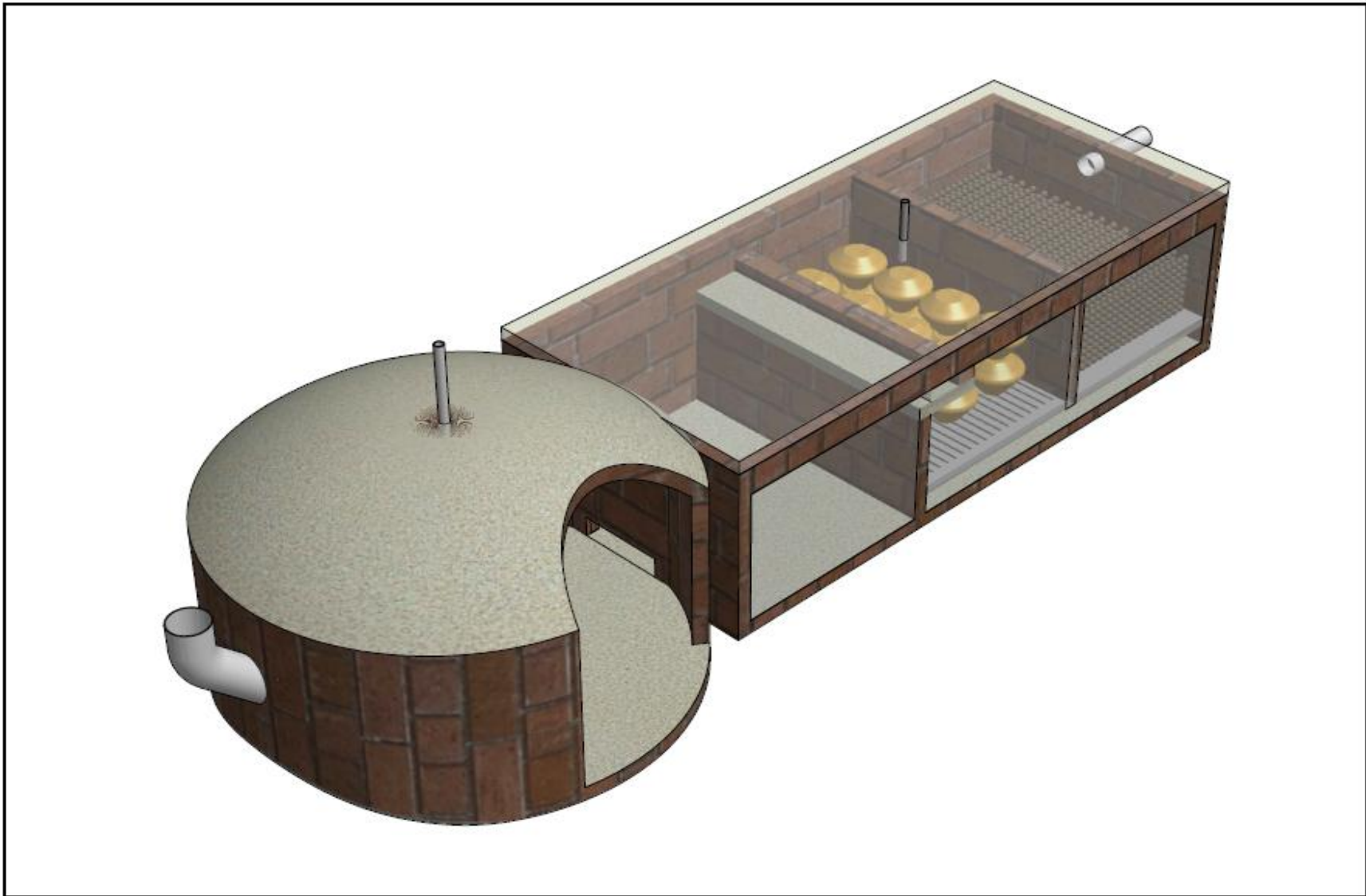
Figure 26: Isometric drawing of the proposed Biogas Septic Tank (Design II)
