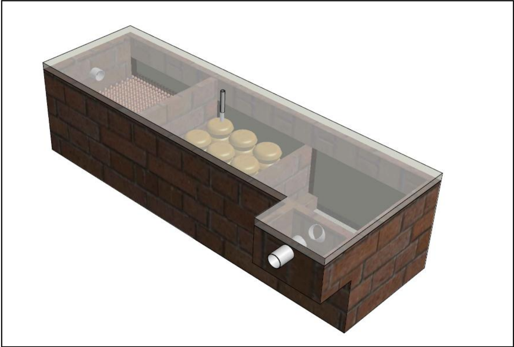
Figure 22: Isometric drawing of the proposed Biogas Septic Tank (Design I)
