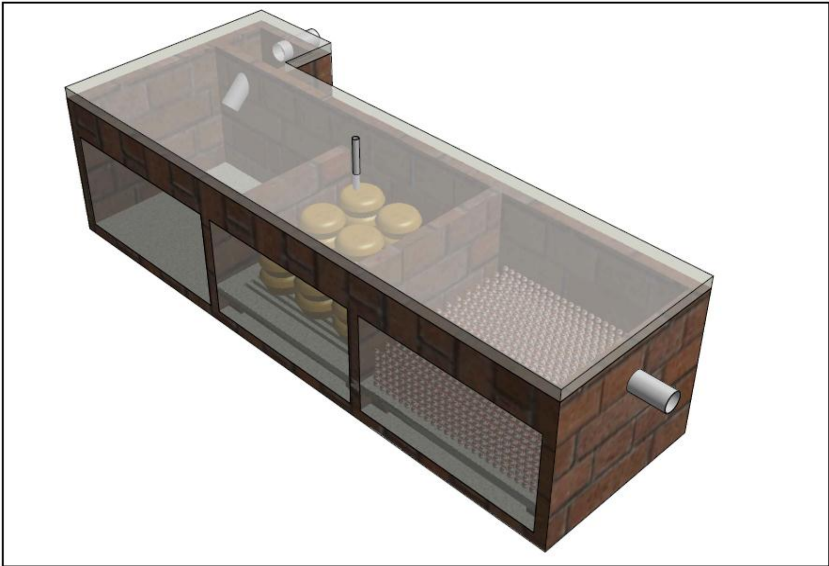
Figure 20: Isometric drawing of proposed Biogas Septic Tank (Design I)
