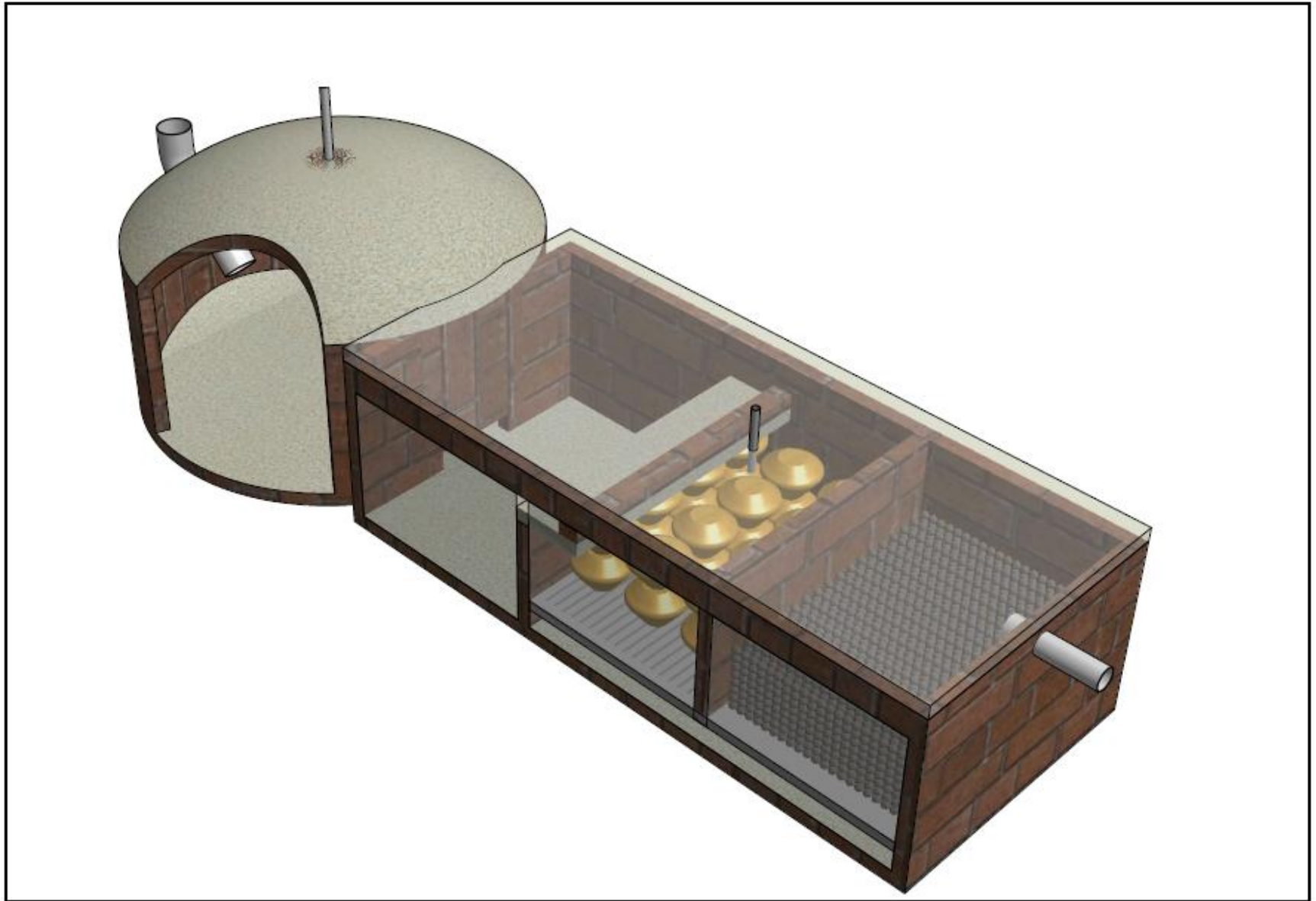
Figure 27: Isometric drawing of the proposed Biogas Septic Tank (Design II)
