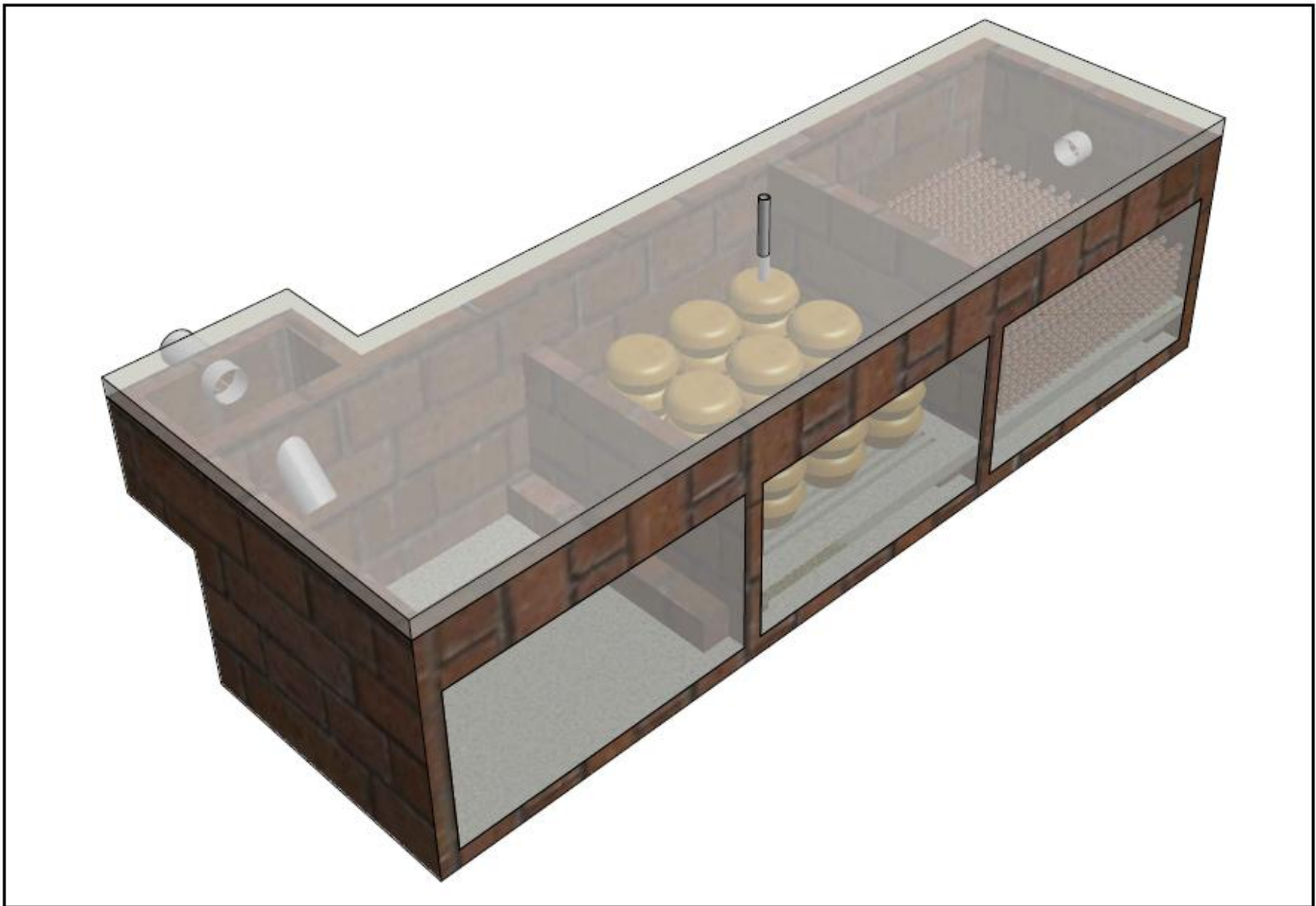
Figure 21: Isometric drawing of the proposed Biogas Septic Tank (Design I)
