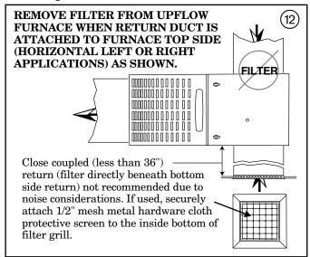
Close coupled (less than 36") return (filter directly beneath bottom side return) is not recommended due to noise considerations.
