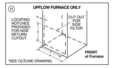
**Downflow Furnaces:** Brackets are factory supplied to mount filters in the return air duct work. When the upflow furnace is installed in the horizontal right or left application and a return duct is attached to the top side as shown in Figure 12, remove the filter from the furnace and install in a remote location.
