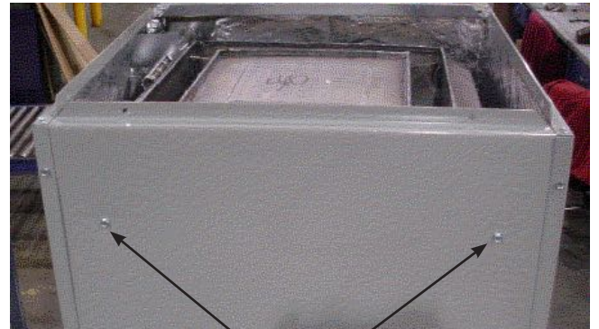
Figure 1 - Heat Exchanger Support Screw Location
