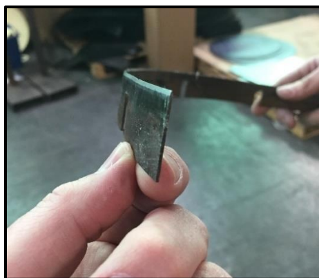
Figure 2-6. Rule Blade for Stamping Machine Photographs courtesy of Branham Corporation and used with Branham’s permission
