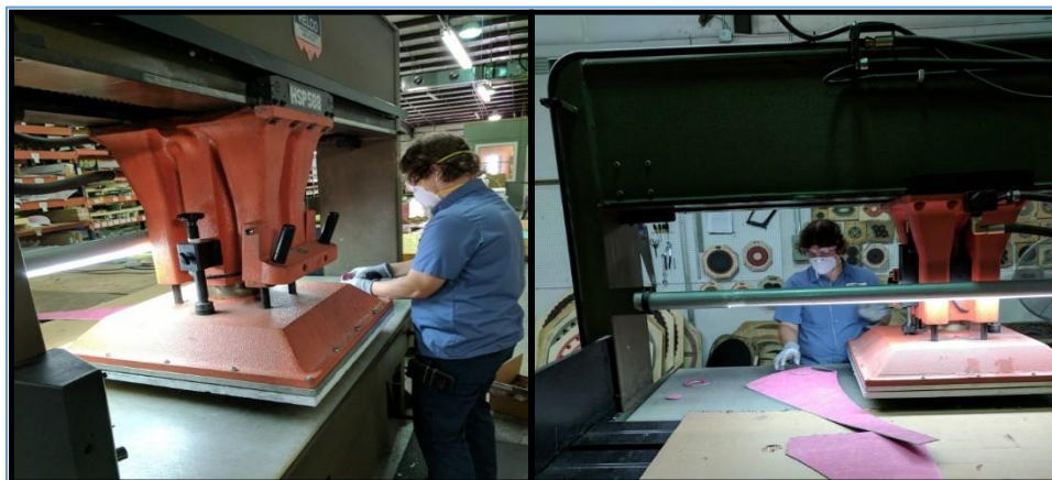
Figure 2-5. Chrysotile Asbestos-Containing Stamping Operation Photographs courtesy of Branham Corporation and used with Branham’s permission
