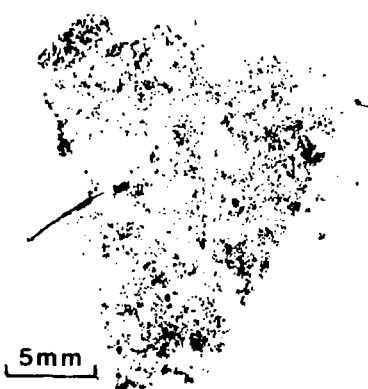
Alpha-radiograph of a weathered sample showing an alpha-particle track pattern from residual uranium decay products
