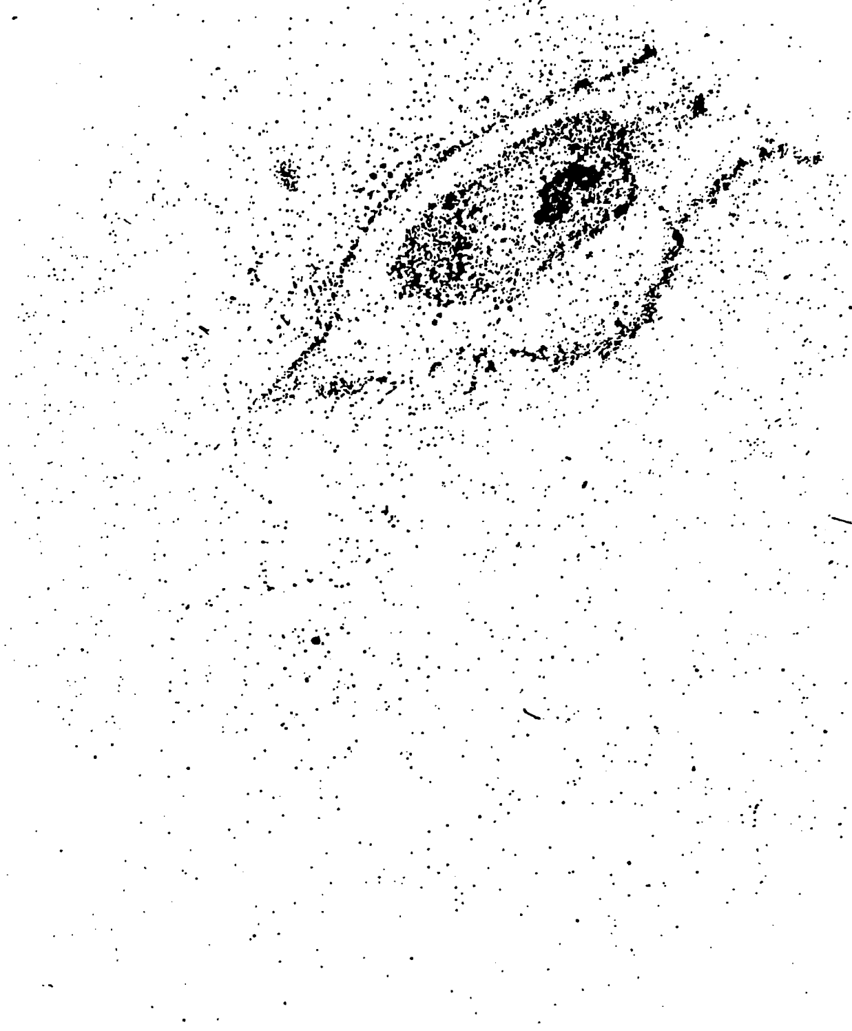
FIG. 9 Large print of an alpha-autoradiograph of a uranium-rich reduction centre in a sandstone. The print shows individual alpha-particle tracks.
