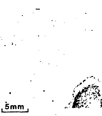
Alpha-radiograph of the same sample with a very well defined alpha-particle source shown in the lower right corner. The upper left source seen in figure 1 does not register on the alpha radiograph since it is beyond the alpha-particle range in rock.
