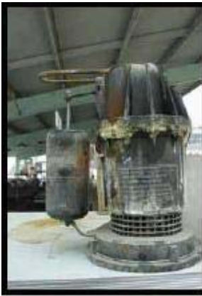
A mercury-free sump pump. Notice the metal guide and no attached wires.
