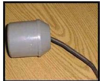
Sump pump float containing mercury.
