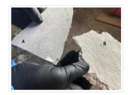
LDB was manufactured from the 1950s to the 1970s as flat and perforated sheet products and was used for wall and ceiling
