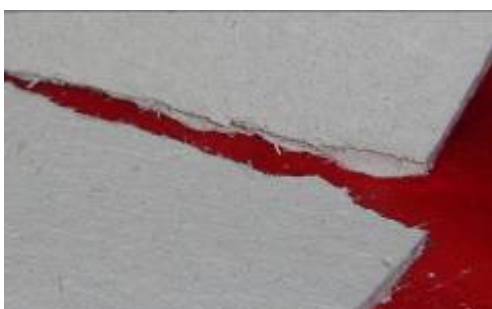
Photos 4 and 5: Ragged or torn edges of broken LDB.
