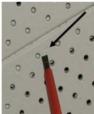
Photo 3: Hand pressure from a screwdriver will dent the surface.
