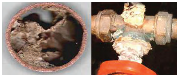
Figure 7.6. Corrosion in Piping Resulting From Galvanic Response
