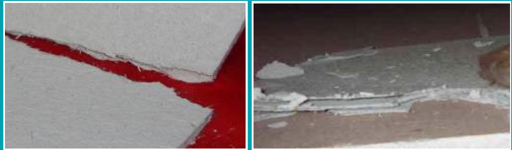
Figure 4 Ragged or torn edges of broken LDB
