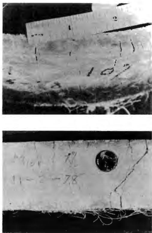
Fig. 8. Multiple cracking characteristics of flexural specimens.
