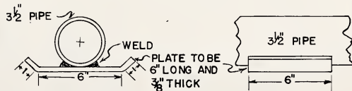
SLIDE PLATE DETAIL
