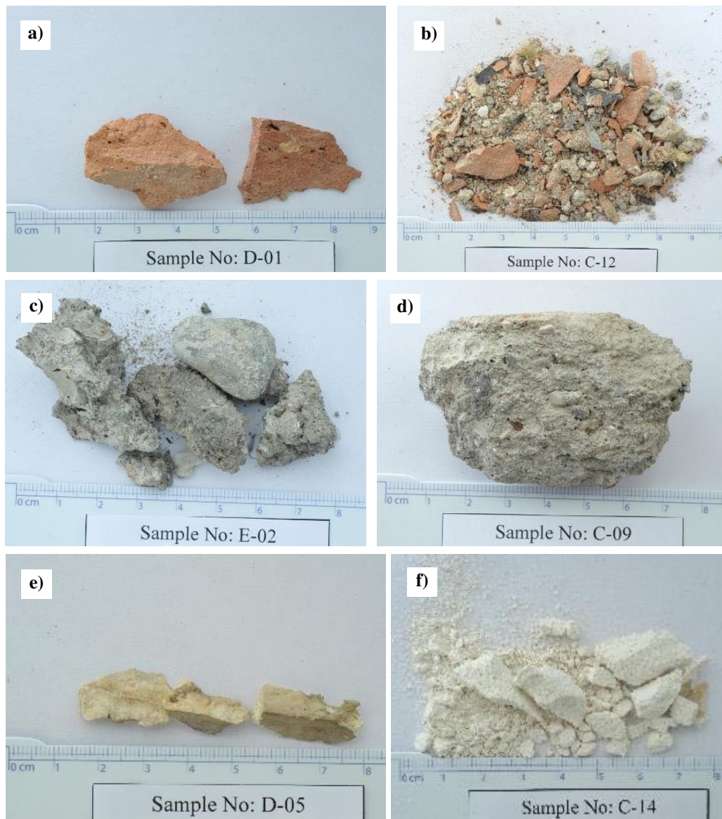
Figure 3.8. Representative macro-photographs of wall materials; a) brick, b) materials fragmented from the main bodies, c) exposed concrete, d) concrete, e) marble, f) plasterboard
