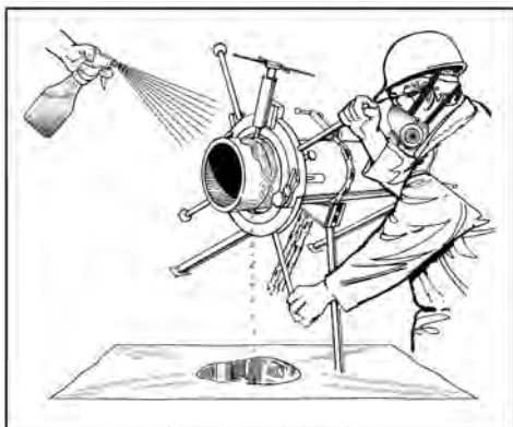
Figure 34-6: Using Manual Pipe Cutter
