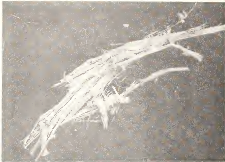
Figure 8. Bulk sample of obviously fibrous tremolite (photomicrograph, 1.8X).
