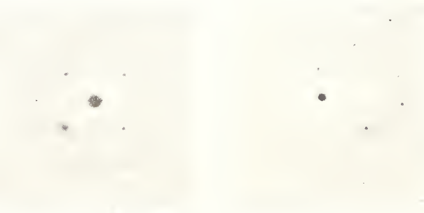
Figure 10. Selected area electron diffraction patterns from two different zone axes in anthophyllite.
