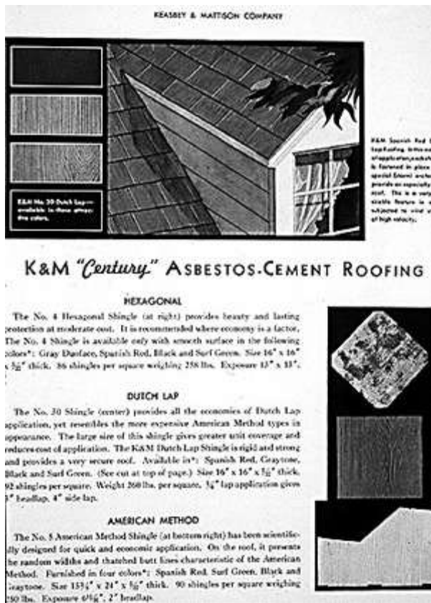
Figure 3. Keasbey & Mattison Company advertisement showing typical asbestos-cement roofing shingles (Sweet's Catalogue of Building Construction, 1940s).
