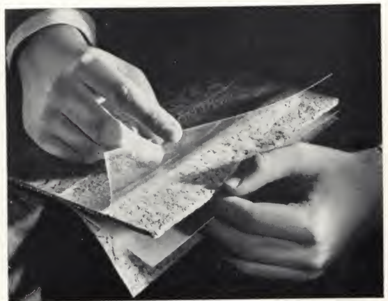
This "exploded" sample shows how the functional value of vinyl is combined with the natural beauty of cork in Custom Vinyl Cork Tile. A layer of clear vinyl is fused to the top and another, located near the back, forms a moisture barrier which makes sure that the tiles won't curl or peak.
