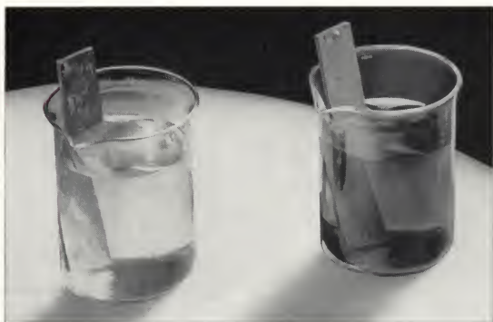
Immersion for 2 hours in a 2 per cent solution of sodium hydroxide determines the color permanency of pigments in tiles specified for use over-, on-, and below-grade concrete. The beaker at the right shows bleeding of colors from pigments that are not alkali resistant.
