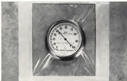
A relative humidity meter, placed under polyethylene sheeting, sealed at the edges with tape or adhesive, should be used on new above-grade concrete before installing materials affected by moisture. After a suitable period, a reading of 80% RH or lower indicates satisfactory dryness.
