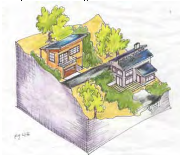
Figure 7-1. Fit development to natural gradient
