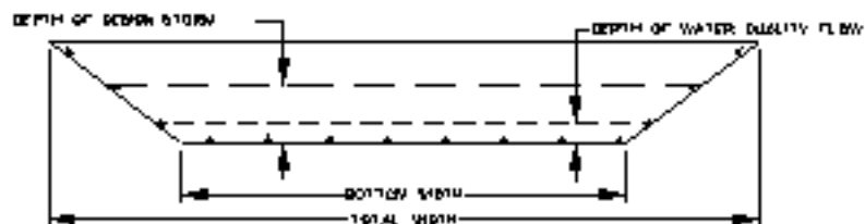
Figure 1 - Diagram of a grassed hydrologic area showing characteristics used in design equations.
