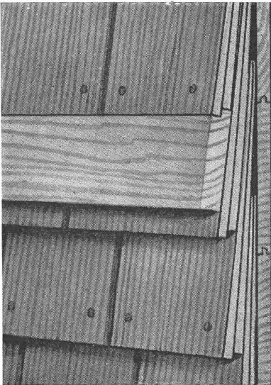
Figure 24. Rabbeted guide for double coursing exterior walls.
