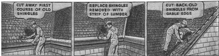
Figure 33. Steps in reroofing.
