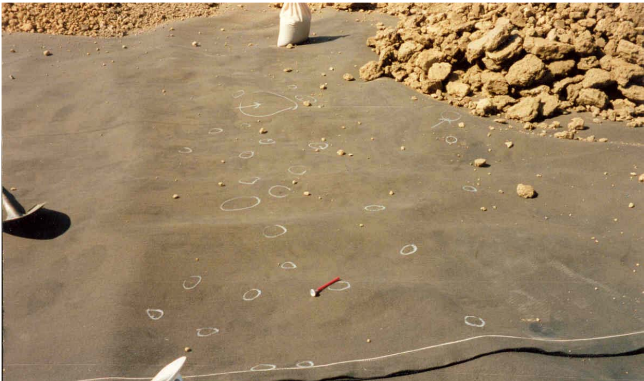
Figure F-A.4.2. Many needle fragments were found in the deployed GT.
