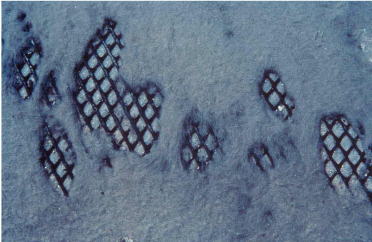
Figure F-A.5.2. Holes developed in a polypropylene GT at the side slope crest after 6.5 months of exposure to the environment.
