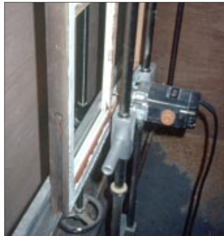
This patented router jig is the core of the Bi-Glass window replacement system.
