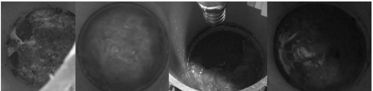
d. Clogging development after the drying period, this sustains for the filters toward the experiment end. Filtration slow down to 3-7 days and scum coverd at the top.
