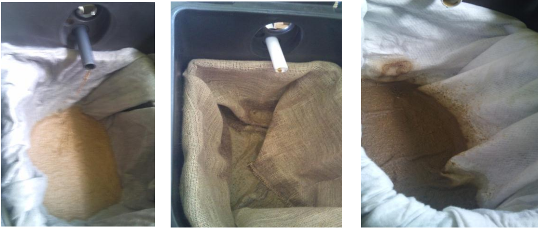
a. Initial loading (both filter1 &3 retain much OM from the very beginning)
