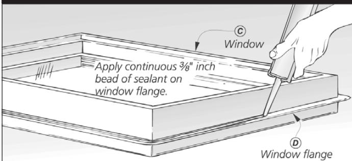
Before installing the window, apply a continuous 3/8" bead of **Moistop® Sealant** to the backside (interior) of the mounting flange. Install the window according to the window manufacturer's instructions.
