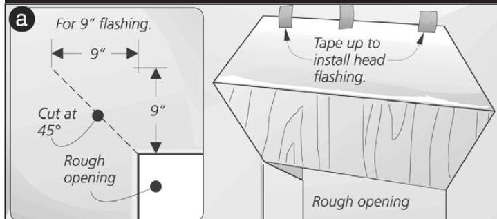
Make the following diagonal cuts at the top of the rough opening corners. Example: for 9" flashing measure as follows: 9" up and 9" over, making a 45° angle (1a). Cut on the diagonal from marked point to the rough opening corner. Gently raise the top edge of the weather-resistive barrier and tape the corners and the center to the barrier surface above. This will allow for the installation of the window and the jamb and head flashing later.
