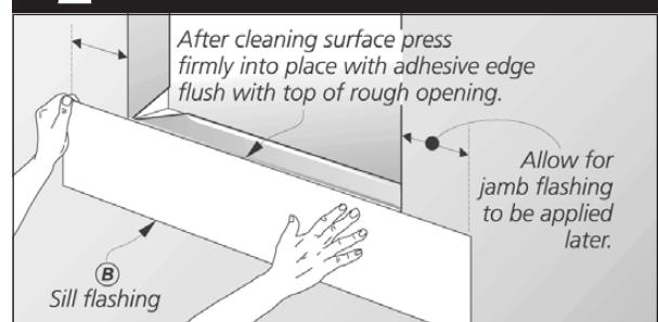
Cut the sill flashing to the width of the rough opening plus twice the flashing width. Wipe the surface of the weather-resistive barrier with a clean rag to ensure proper adhesion. Remove the release paper and press the sill flashing in place so that the edge of the flashing's adhesive is level with the top edge of the rough opening.
