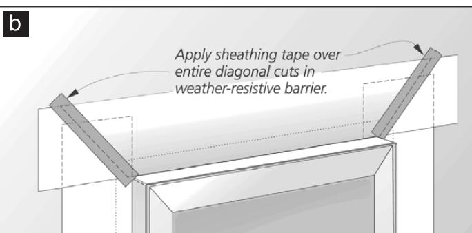
Finally, allow the flap of the weather-resistive barrier at the head to lay flat over the head flashing. Apply a new piece of sheathing tape over the entire diagonal cut made in the weather-resistive barrier and press firmly in place.
