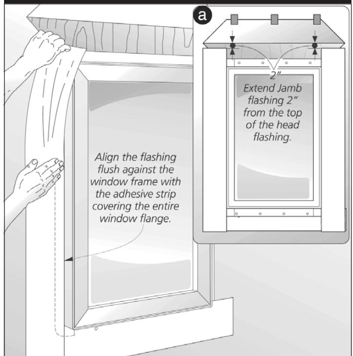
Prior to installing the jamb flashing wipe the jamb flange and weather-resistive barrier with a clean rag to ensure proper adhesion. Then cut two strips of flashing long enough to extend beyond the sill flashing and 2" below the top of the head flashing. Remove the release paper and align the flashing flush against the window frame with the adhesive strip covering the entire window flange. Follow this procedure for the other side of the window.
