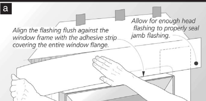
Wipe the head flange, jamb flashing, weather-resistive barrier, and sheathing with a clean rag. Cut a piece of flashing long enough to ensure that the head flashing extends a minimum 1" beyond the jamb flashing. Install the head flashing by pressing firmly in place in one direction to prevent voids.
