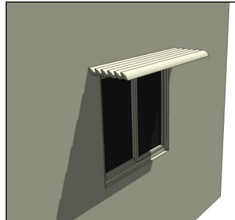
Figure 4b: Sunscreen used horizontally in place of overhang for more diffused light while still shading.
