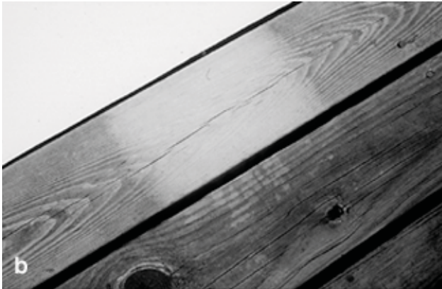
Figure 7—Removal of mildew from lumber treated with chromated copper arsenate (CCA): (a) mildew-infected board; (b) mildew removed with a bleach-water solution.
