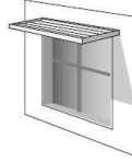
Use louvers in place of Solid overhang for more diffuse light while still shading.
