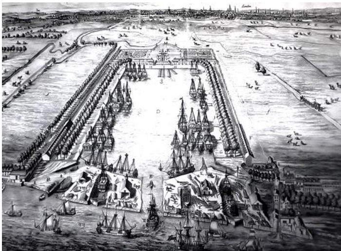
Figure A.1. Howland Great Wet Dock (drawn 1717, though originally constructed 1696). The basin was sheltered by deliberately planted trees along the quaysides. Note the two small dry docks either side of the entrance to the basin. These have lock gates whereas the main basin does not. It is probable that the water level in the main basin was maintained by a cill. There were no warehouses.
