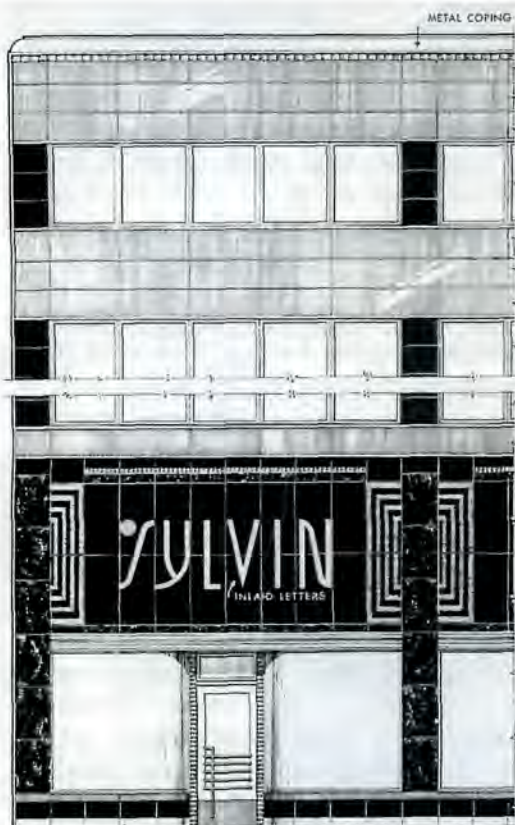
VITROLITE EXTERIOR TREATMENT OF BUILDING STORE FRONT SHOWING CURVED BULKHEADS AND SANDBLASTED DECORATION. VITROLITE FOR UPPER STORIES HELD IN PLACE BY MASTIC CEMENT AND METAL MOULDINGS. SCALE 1/4"=1'-0"
