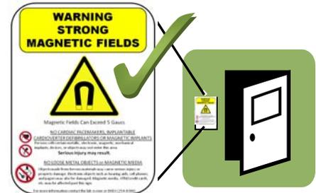
In addition to the warning signs posted at the doorways, some method to indicate the 5 gauss line around the magnet is required. For example, a painted line or tape placed on the floor around the magnet where the field is 5 gauss could be used. Another example is a chain, rope, or fence indicating the 5 gauss line around the magnet. Whatever method is used, egress from the area in the event of an emergency shall not be blocked or prevented.
