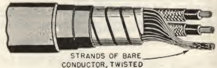
Fig. 7-9. In service entrance cable the neutral wire is not insulated, but is bare, and wrapped spirally around the insulated wires. The picture shows 3-wire cable.
