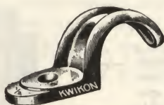
← Fig. 7-13. Entrance cable should be anchored to the building every 2 ft. Use straps of the type shown.
