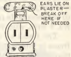
Fig. 15-3. Plaster ears are helpful in aligning a device flush with the plaster.
