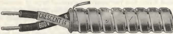
Fig. 10-1. Armored cable consists of two or three Type R or Type T wires, protected by a layer of tough paper and flexible galvanized steel armor. Fig. 10-2. Staple for cable.
