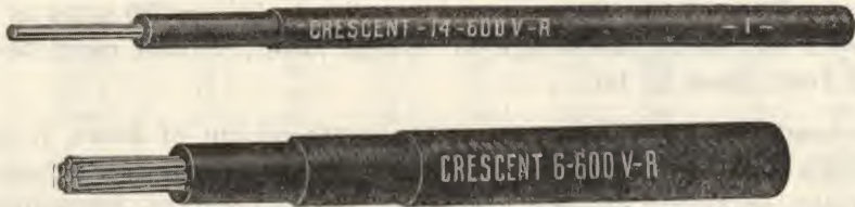
Fig. 4-4. Rubber-covered wire is usually used only indoors. If it is No. 6 or larger, the conductor is stranded and there are two cotton braids, as shown in the lower picture.
