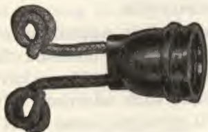
Fig. 16-14. A weatherproof socket makes an excellent test lamp.
