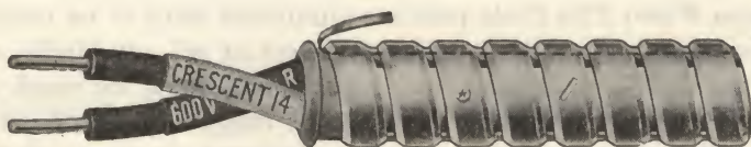
Fig. 4-6. Armored Cable consists of two or three individual wires, assembled into a cable, protected by flexible steel armor. It may be used only indoors.
