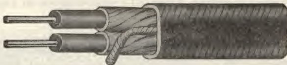
Fig. 4-5. Nonmetallic Sheathed Cable consists of two or three individual wires, assembled into a cable. It may be used only indoors. Code Type NM is shown. Type NMC is shown in Chap. 17.
