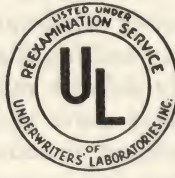
Fig. 1-2. Some approved merchandise is not so marked, but the tag or carton bears one of the markers at left. "UL" means "Underwriters' Laboratories."
