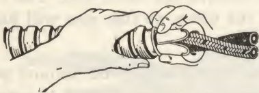
Fig. 10-8. Insert the bushing between wires and armor.
