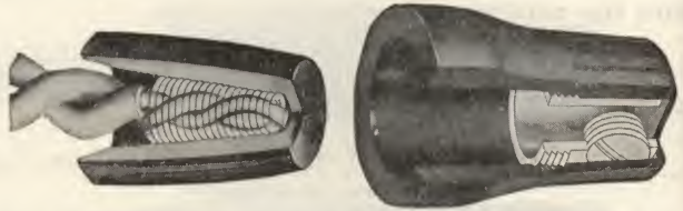
Fig. 4-15. Solderless connectors save a great deal of time, as compared with soldering. No taping is necessary.
