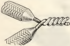
Fig. 4-14. If there is no strain on the wires, merely twist them, solder, tape.
