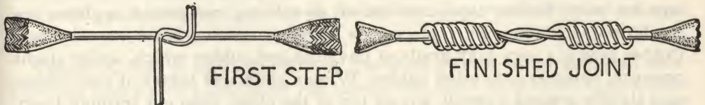
Fig. 4-20. When there is strain on the wire, splice as in picture above.
