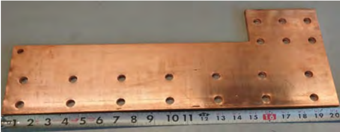
Figure 4 Copper Bus Bar Extension
