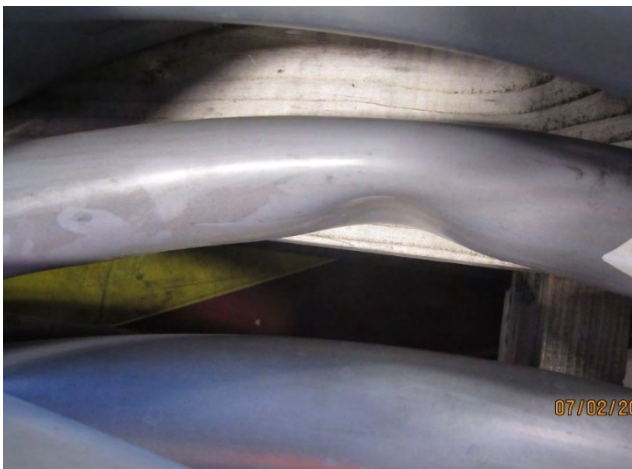
Figure 3. Defect: Large Dent
