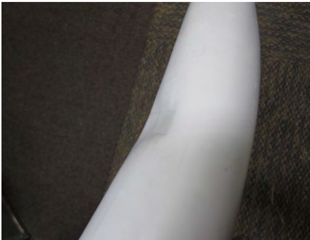
Figure 1. Defect: Small Dent
