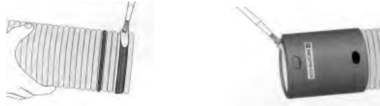
Figure 22 Key-Lock™ Couplers Lubricant Application
