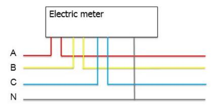
**Live/Load line:** There will generate voltage (100 ~ 240V) between A/B/C line and N line, we call A, B and C line live/load line.
