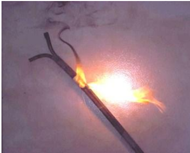
Fig. 13 Smoke and flames originating from the area of fiberglass tape.
