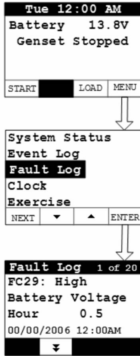
FIGURE 27. FAULT LOG SCREEN
