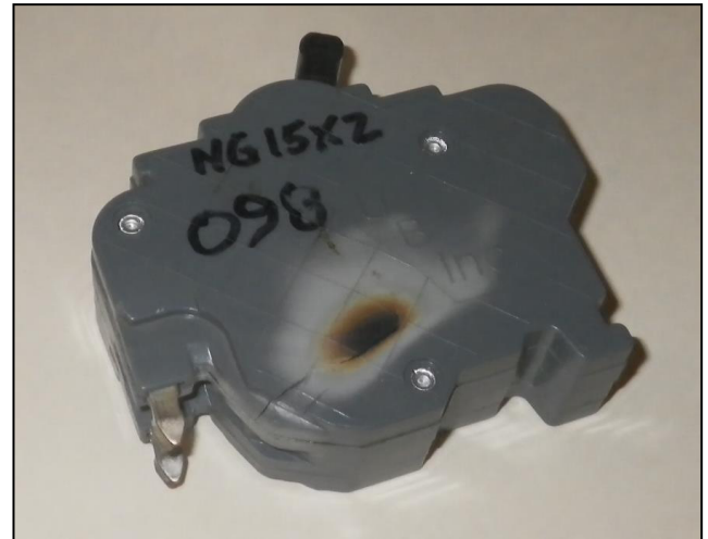
FIGURE 8. Brand 10 (X) 15A 2-Pole Breaker, Jammed, Tested to 60A.
