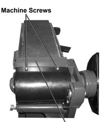
Fence (63) Tabs (not shown) are underneath Belt End Guard (58) where Machine Screws are shown. Figure F
