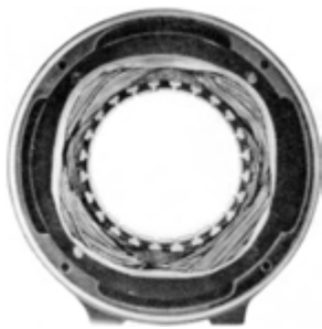
Fig. 2-11: Typical four-pole, split-phase stator.
