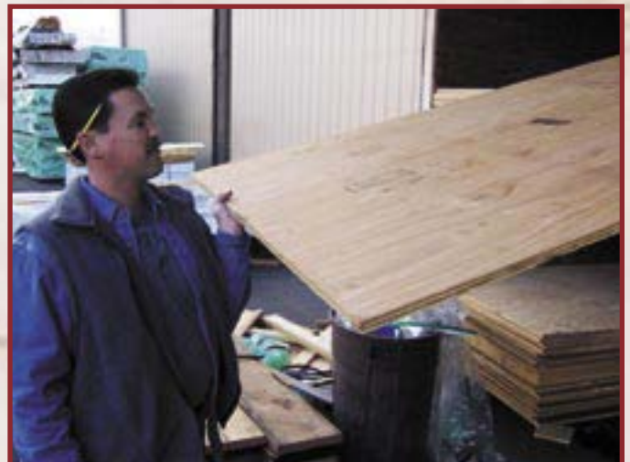
Figure Two: Inspecting plywood for fire-rating.
