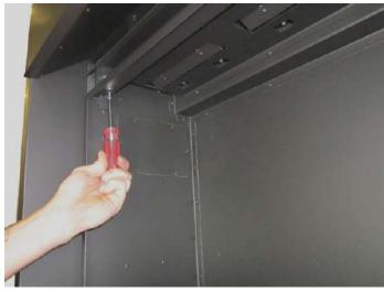
The side fireback clip has a keyhole slot. It can be removed by loosening the screw and sliding the clip out.
