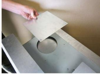
2 Remove the 2 screws on the outer cover plate and remove the cover.
