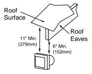
E Minimum 11" (279mm) clearance below unventilated soffits or roof surfaces
