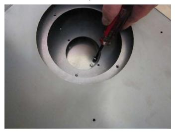
5 Rotate the convection cover plate 180° (this allows heated air to flow upwards into the power heat duct).
