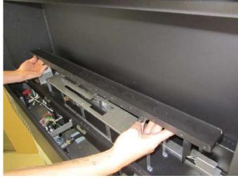
4. Remove the burner support as shown below. It is held in place with 6 screws (1/4" nutdriver) and 4 nuts (11/32" nutdriver).
