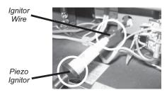
Disconnect the ignitor wire from the Piezo Ignitor and connect it to the DC Sparker.
