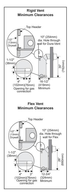
6) Use steel studs for framing where the 1-1/2" (38mm) clearance from the vent to combustible material cannot be maintained.
