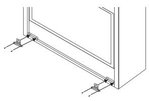
6) Place the Bottom Frame near the hinges, and flip down the hinges from the Bottom Face Plate. Secure the hinges in place to the Bottom Frame, using 2x #8 Self Tapping Phillips screws per hinge.
