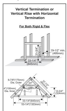
**NOTE:** If this is an outside corner, the minimum distance between the vent and the outside corner is 6" (15cm) with AstroCap termination cap or 12" (30cm) with Rigid Vent termination cap. (For example Dura-Vent).
