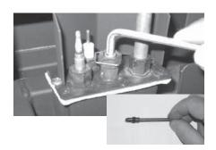
Remove burner orifice with a 1/2" wrench and discard. Use another wrench to hold on to the elbow behind the orifice.
