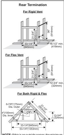
**NOTE:** If this is an outside corner, the minimum distance between the vent and the outside corner is 6" (15cm) with AstroCap termination cap or 12" (30cm) with Rigid Vent termination cap. (For Example Dura-Vent).
