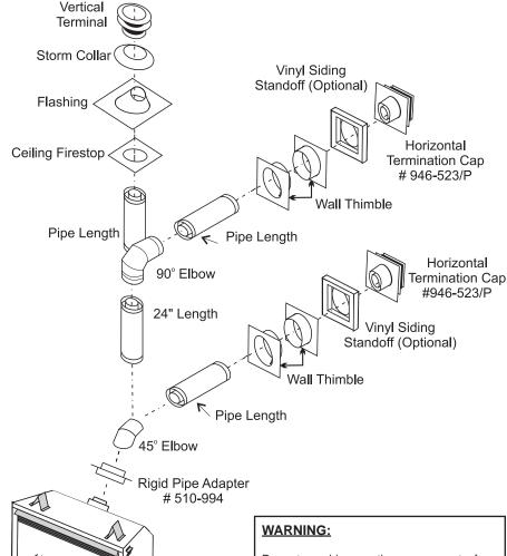
Do not combine venting components from different venting systems.
