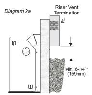
Below Grade Snorkel Installation If the Snorkel Termination must be installed below grade, i.e. basement application, proper drainage must be provided to prevent water from entering the Snorkel Termination. Refer to Dura-Vent Installation instructions for details. Do not attempt to enclose the Snorkel within the wall, or any other type of enclosure.
