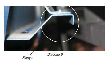
6) Hook the flange on the faceplate over the top of the flush door and gently lower the faceplate into place until it rests against the faceplate supports as shown in Diagrams 7 & 8.
