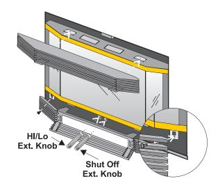
6) Open the bottom louver. Pull the Burner ON/OFF control box from inside the bottom of the fireplace and position the slots in the bracket over the 2 screws on the left side of the bottom louver. Push down to lock into place. Tighten the screws.
