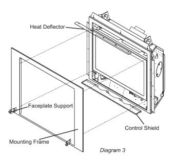
3) Loosen 4 phillips head screws located inside firebox, for screw locations see Diagram 4. Install mounting frame and retighten screws.
