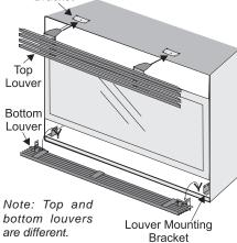
Open the bottom louver. Pull the Burner ON/OFF control box from inside the bottom of the fireplace and position the slots in the bracket over the 2 screws on the left side of the bottom louver. Push down to lock into place. Tighten the screws.
