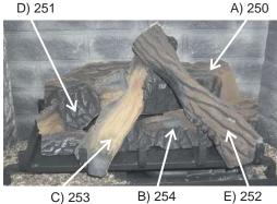
4) Place Log 254 on the front right side of the burner. Push the back of the log against the 2 brackets with the notch on the bottom right side of the log fitting into the right side of the grate.
