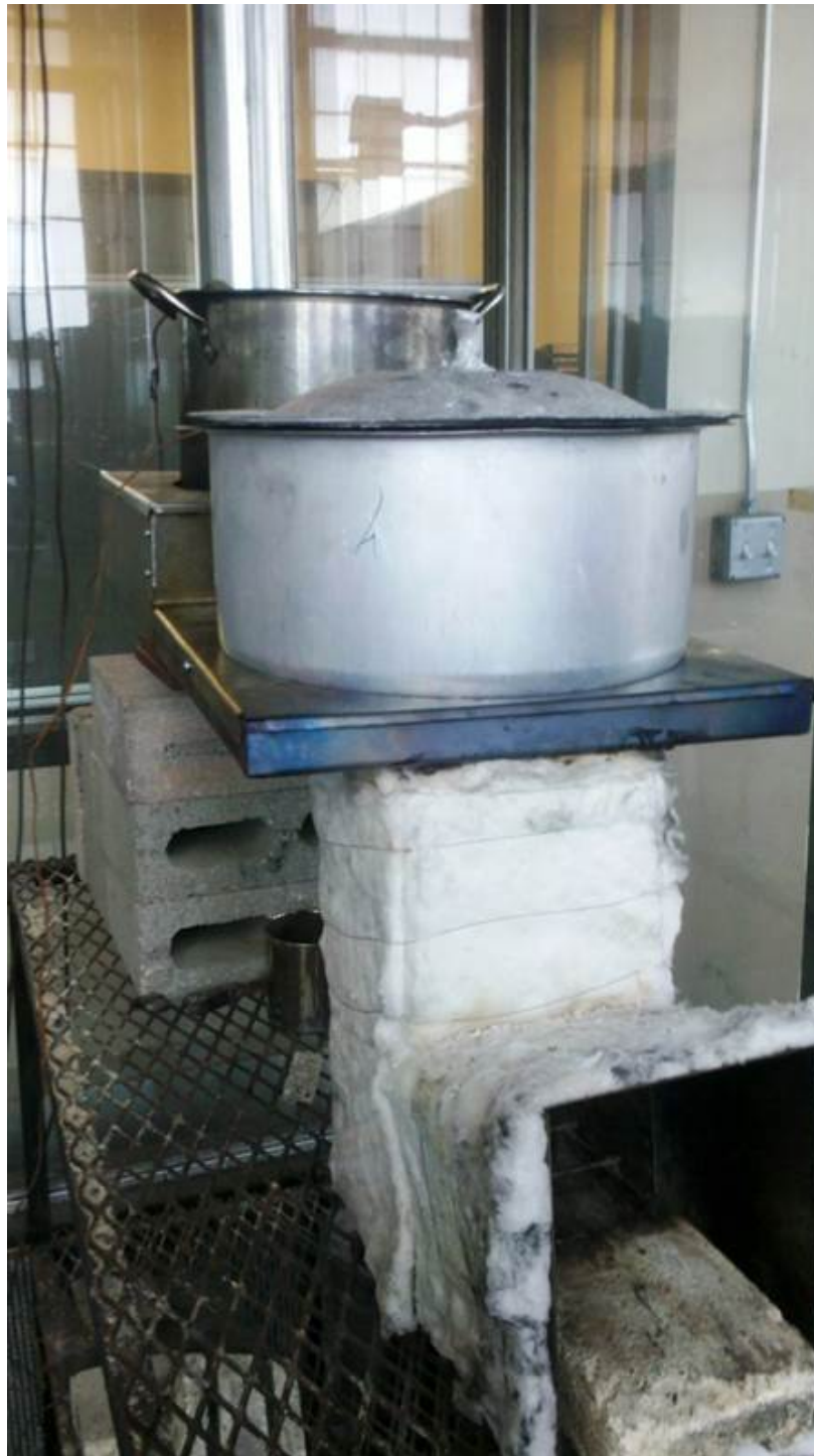
FIGURE 28. The L60460, a two-pot experimental prototype stove developed as part of this work.
