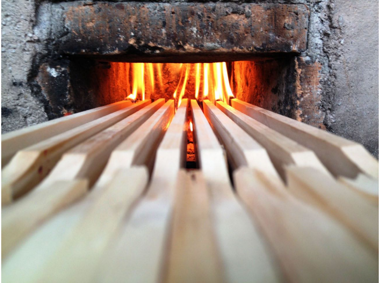
FIGURE 24. Fuel bundles made from precisely spaced wooden shims allowed for regulation of stove firepower.
