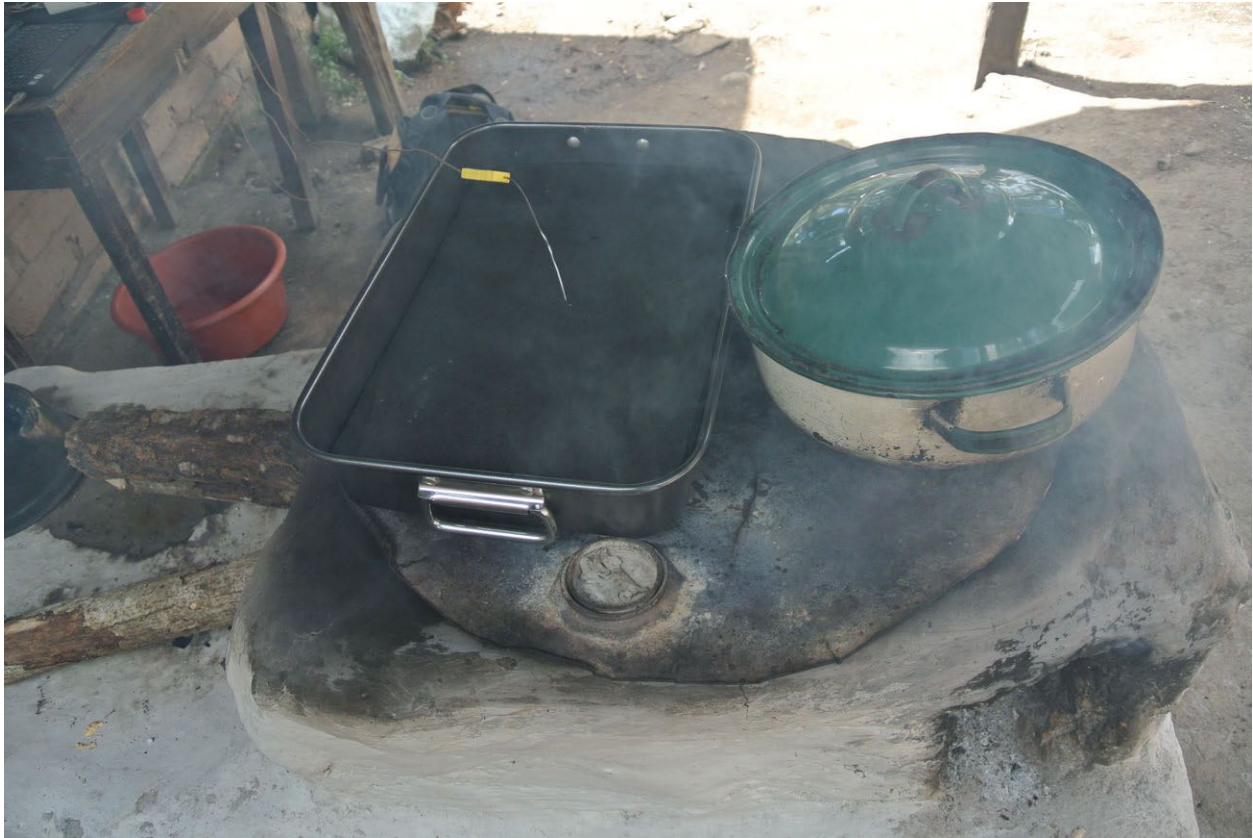
FIGURE 5. Traditional plancha stove in Valle de Ángeles, Honduras. Construction typically consists of 3 blocks, covered with cement, with a steel oil drum top.
