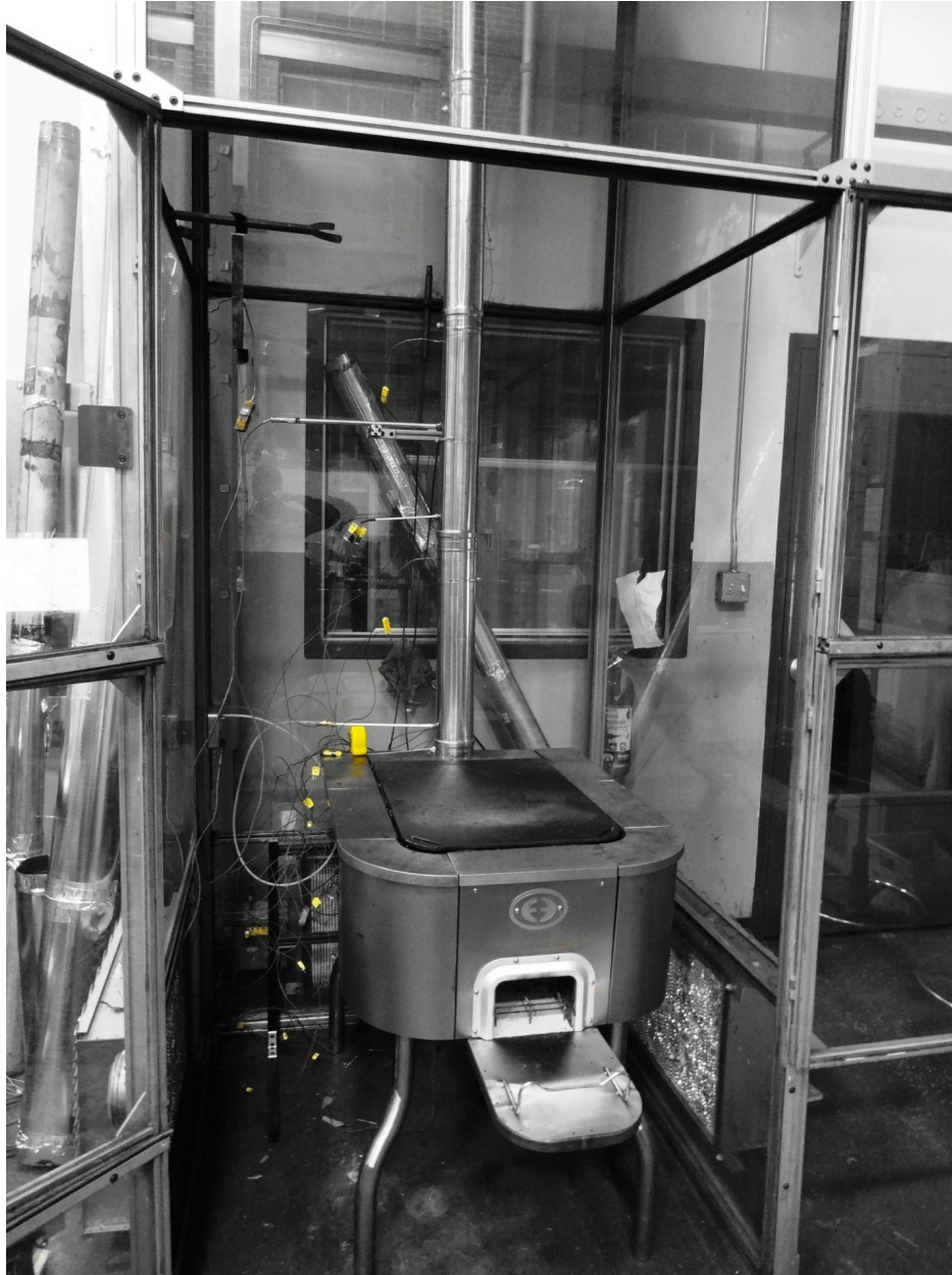
FIGURE 26. The HM5000 plancha stove, developed as part of this work was tested extensively.
