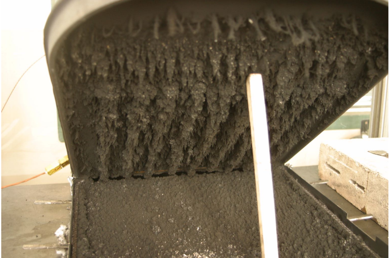
FIGURE 64. Use of pitchy pine in previous version of the HM5000 after several hours of use
