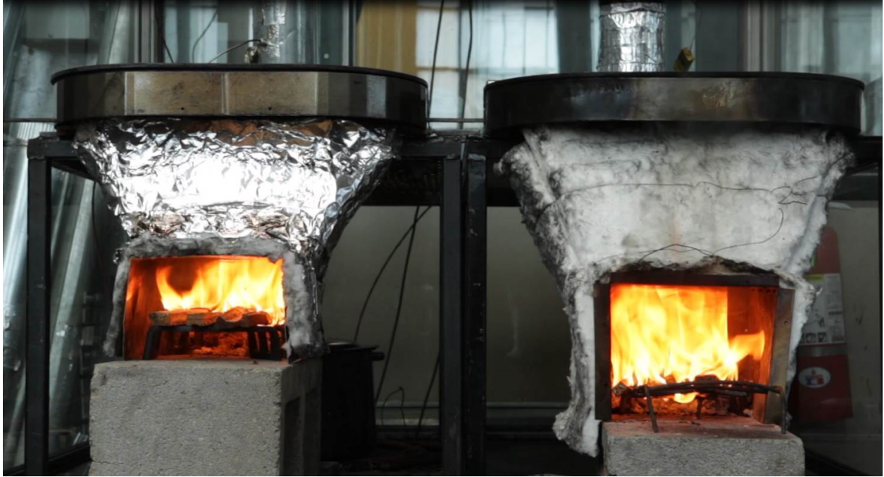
FIGURE 56. Frontal velocity was increased by decreasing the cross sectional area of the combustion chamber inlet.
