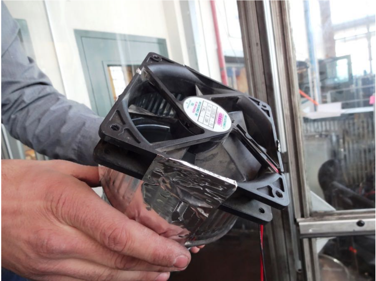
FIGURE 29. Powered fan installed on top of chimney for natural convection equivalence testing.
