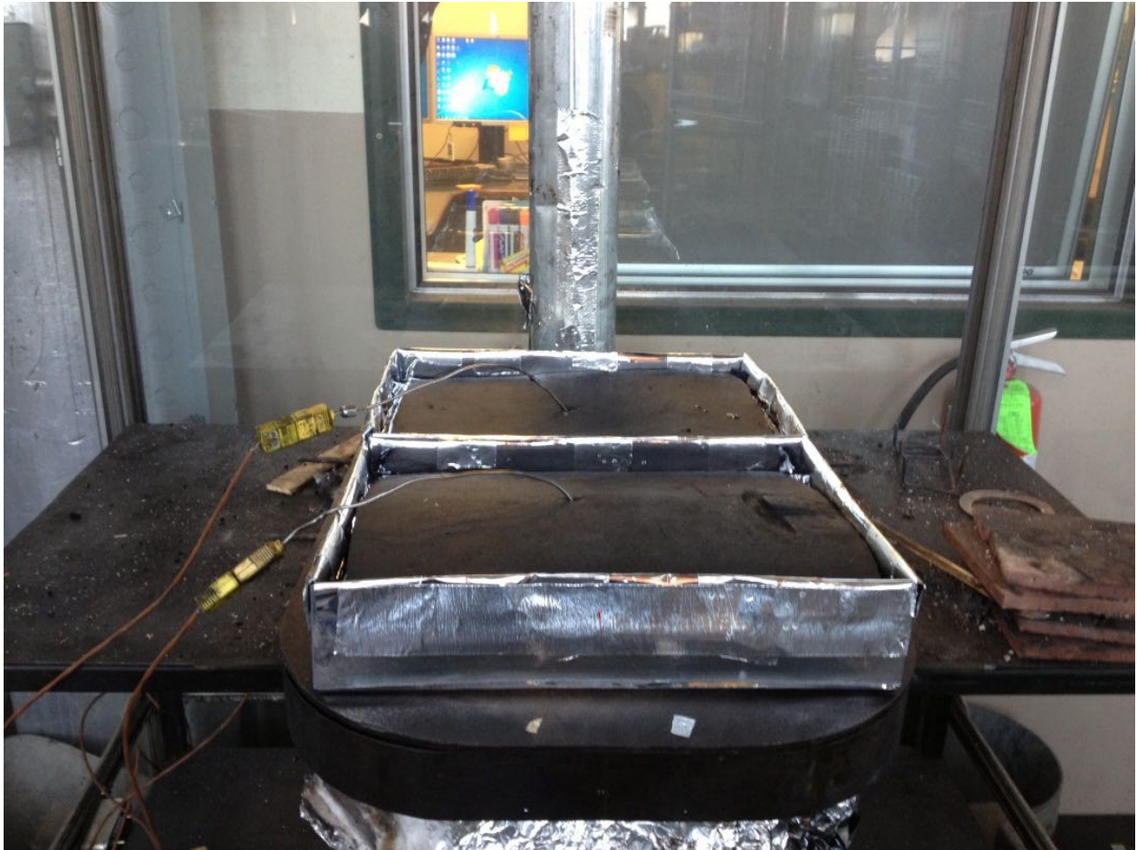
FIGURE 32. Flexible-bottom pots were constructed and used for testing as part of the griddle testing protocol.
