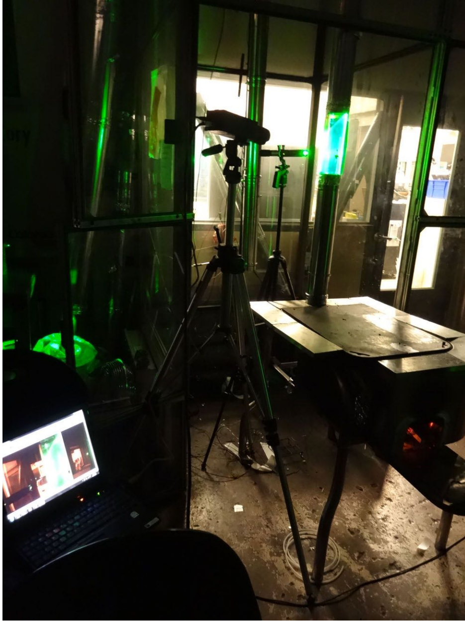
FIGURE 20. Rudimentary Particle Image Velocimetry (PIV) setup used to validate the high temperature hot-wire anemometer
