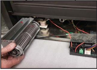
. Slide the blower along the back wall until it reaches the stop flange, then feed the blower wires underneath the gas supply to the front as shown.
