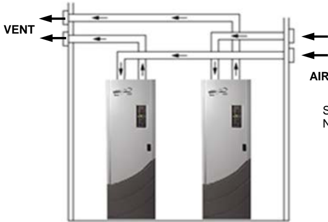
Individually Sealed Combustion Located on Different Wall From Exhaust
