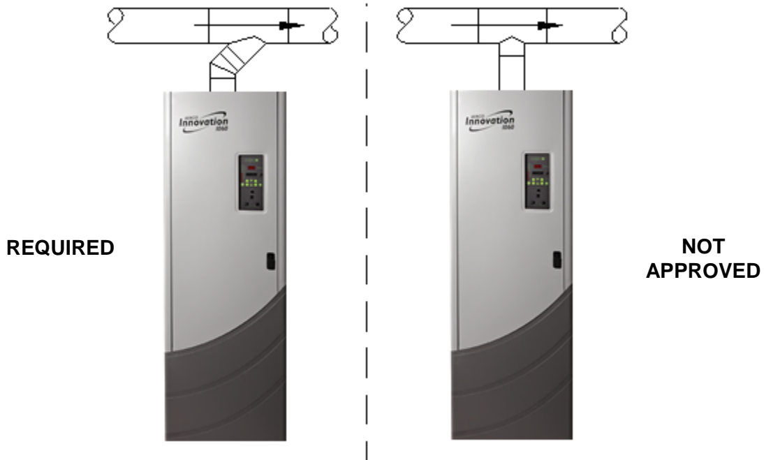
Figure 11a: Recommended Connections to Common Vent Breeching
