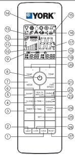
1.CODE Used to select CODE A or B which will be displayed on LCD.Please select A without special explanation. 2.LIGHT button Control the lightening and extinguishing of the indoor LED display board. 3. TIMER button 4. CLOCK button 5. SLEEP button 6. TIME button
