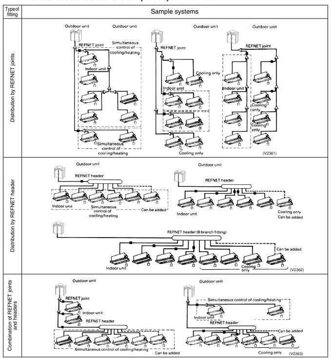
Units can be added by connecting them directly to the REFNET header or REFNET joint. Further branches cannot be included in the system below the REFNET header branch.
