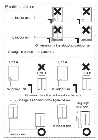
3. If the connecting pipe length between outdoor units exceeds 80 inches, it is necessary to install a vertical loop in the gas line at least 8 inches in height and not more than 80 inches from the main outdoor unit closest to the first connected indoor unit. See following diagram:
