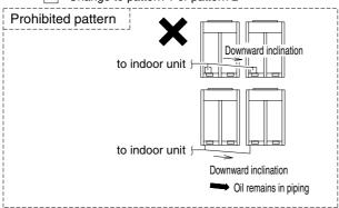
2. To avoid the risk of oil retention to the end unit, always connect the stop valve and the piping between outdoor units as shown in the figure A or figure B.
