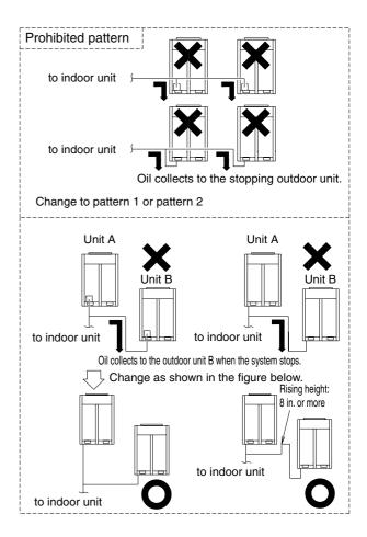
3. If the piping length between the outdoor unit-connecting pipe kits or between the outdoor units exceeds 80 in., create a rise of 8 in. or more in the gas line within a length of 80 in. from the kit.
