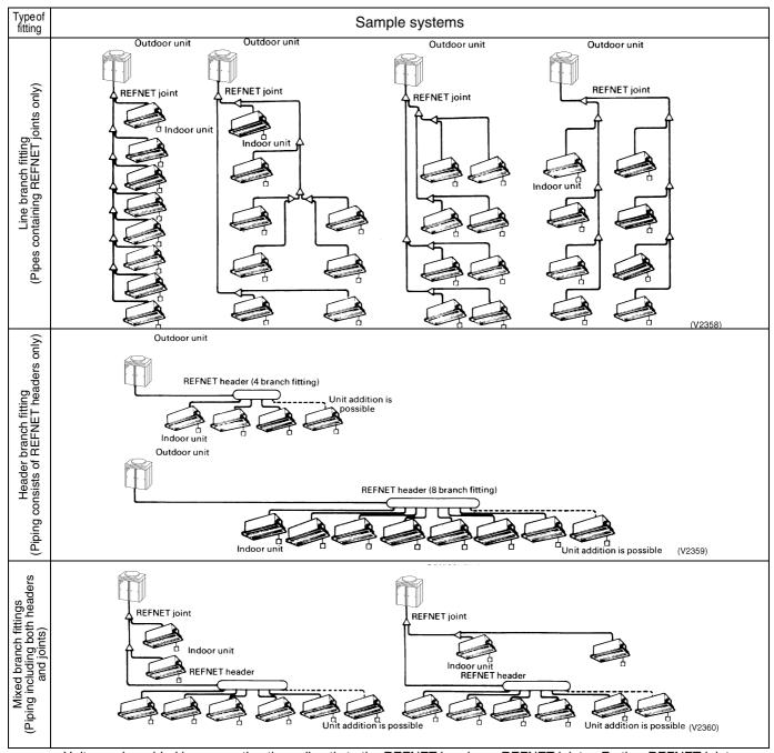
Units can be added by connecting them directly to the REFNET header or REFNET joint. Further REFNET joints cannot be included in the system downsteam of a REFNET header.
