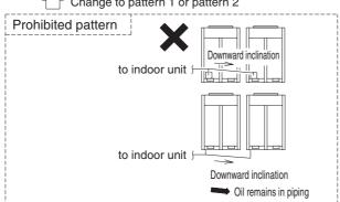
2. To avoid the risk of oil retention in the stopping unit, always connect the stop valve and the piping between outdoor units as shown in the figure A or figure B.
