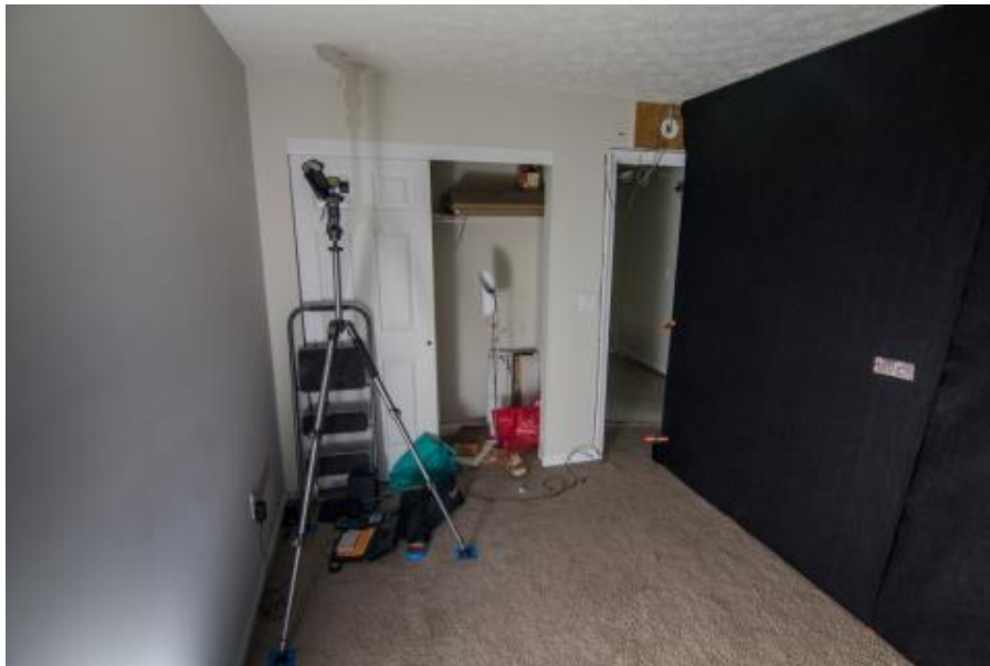
Figure 15. Wide-angle IR camera (left) facing black felt IR viewing screen positioned adjacent to a wall and parallel to the primary register airflow path
