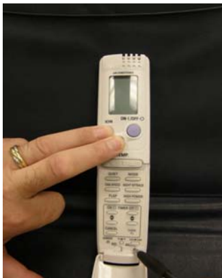
With a pen press the ACL button down while holding the ION and 1 Hour Timer buttons down
