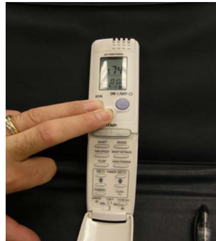
Using two fingers hold the ION and 1Hour Timer buttons down together
