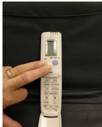
Release the ACL button first then release the ION and 1 Hour Timer buttons
